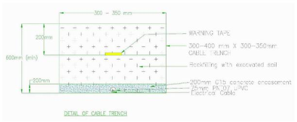
It is necessary to Provide additional length (about 100mm) of every cable near each and every junction box for future use. All the cables lay across pathways and roads shall be laid in 110mm dia. PNT07 grade uPVC ducts with concrete encasement.
