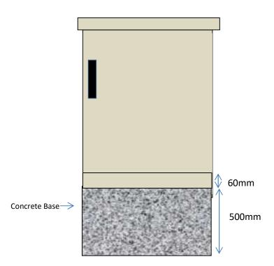
This panel shall complete with all its internal switch gear and control devices with wiring as per the given drawing. Load wires shall be arranged to connect the system with main DB. **Dimensions of the panel shall be decided by the panel builder & 20% additional space shall be provided.**
