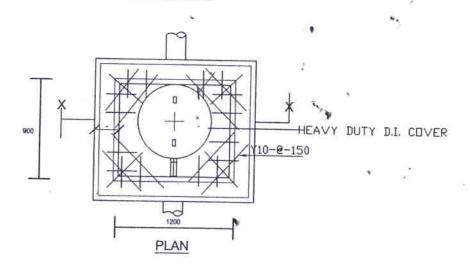
1. ALL DIMENSION ARE IN MILLIMETERS. 2. DISTRIBUTION STEEL AT T10 € 200 mm c/c
